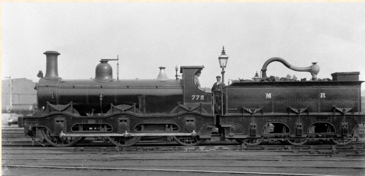
A driver and fireman in the cab of a Kirtley Class 700, built between 1869 and 1874. It is seen here before 1907 when the Midland's numbering system was changed. As a fireman in the 1870s, and as a driver from 1889, Thomas would have been familiar with these locomotives. (Mick Hymans Collection, with thanks to Charlie Verrall )
